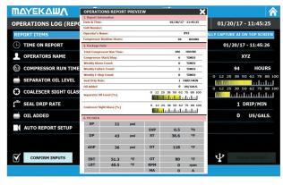
The MYPRO TOUCH+ also offers options to remotely monitor the HMI from a smart phone or tablet. Combine this feature with a VPN access to your network and you can have 24/7/365 access to your MYPRO TOUCH+. Simply download a VNC viewer app to your smart device and connect to the IP address of your MYPRO TOUCH+ panel in your network.
